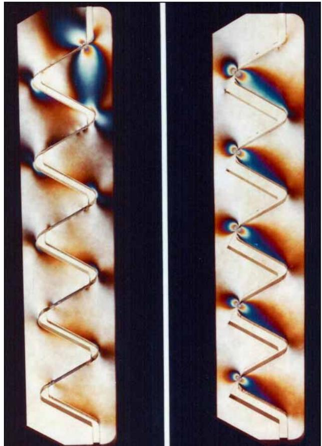
*Photoelastic comparison of Spiralock’s 30° wedge ramp (right) shows distributed threaded joint’s load throughout all engaged threads. The first two threads on the conventional thread (left) often carry as much as 80% of the load, enough to cause shearing or stripping.*
